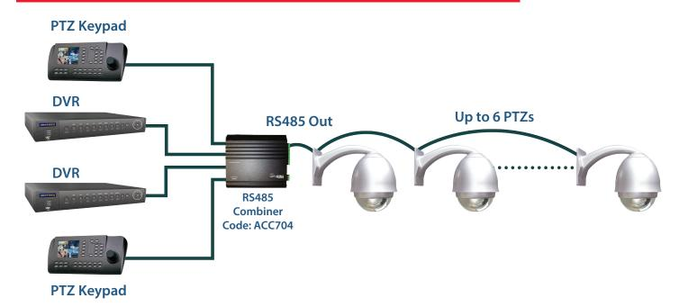
This RS485 combiner allows you to connect up to four RS485 inputs from controllers such as DVRs, Keyboards and Matrix units. All four inputs can be activated at the same time and each input device can have any protocol, baud rate and ID.
